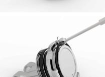
• Remove the piston guide bushings (pos. 13). This can be done by twisting them out of their groove.
