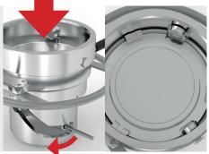
• Remove the inner package by pressing the piston guide from behind. If the driving plate does not loosen easily use a soft tool, e.g. made by rubber, and carefully press the driving plate out.
