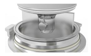
Reasemble the piston o the piston guide, make sure that the splint (pos 63) is correct mounted.
