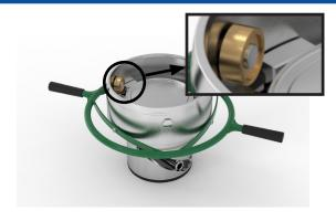
Turn the driving plate to the position where the driving plate heels are coming free from the rollers. It could be necessary to release the package from the press force.
