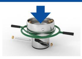
Remove the shaft and rollers (pos 15 & 16) for piston guide, by applying slight pressure to the driving plate package so that it moves down, until the driving plate package is released from the rollers.
