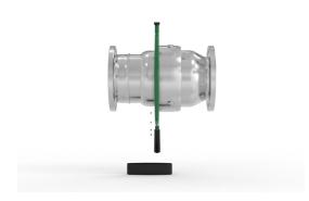
Put a small container underneath the coupling and start twisting the svivel sleeve, so the balls drop out, into the container. Placing a tank unit in the hose unit will make it easier to twist. Save the 77 balls for reassembling later.
