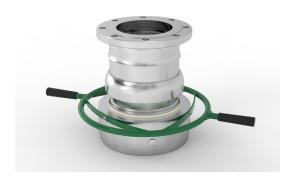
Remove the swivel sleeve by pulling out the hose unit body with the inner package. If the swivel sleeve cant be removed, there might be some balls left inside. Try turning back and forth again to get out the remaining balls.
