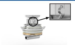
Dismounting the inner package by removing the pin and splint (pos 5 & 63) from the piston. Remove all parts from the inner package in order to change the seals (pos 8 & 77) on the driving plate and the seal (pos 3) on the piston.
