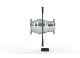
Put a small container underneath the coupling and start twisting the svivel sleeve, so the balls drop out, into the container. Placing a tank unit in the hose unit will make it easier to twist. Save the 59 balls for reassembling later.
