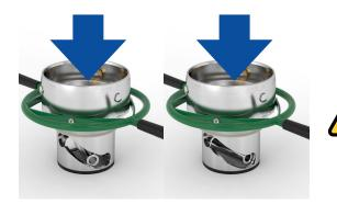
Assemble the shaft and two rollers for piston guide by applying pressure to the driving plate packet.
