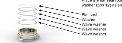
Place the flat seal (pos 29), washer (pos 14) and wave washer (pos 12) as shown in the picture.
