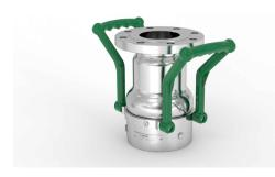
Use Loctite® 243 and screw the lock screw (pos 23) and o-ring (pos 78) into the swivel ring without any force! Risk to deform the ball bearing!
