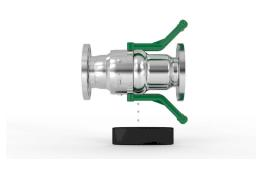
Put a small container underneath the coupling and start twisting the svivel sleeve, so the balls drop out, into the container. Placing a tank unit in the hose unit will make it easier to twist. Save the 59 balls for reassembling later.
