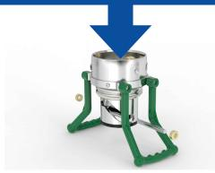
Remove the shaft and rollers (pos 15 & 16) for piston guide, by applying slight pressure to the driving plate package so that it moves down, until the driving plate package is released from the rollers.
