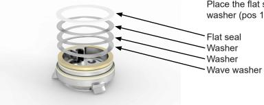
Place the flat seal (pos 29), washer (pos 14) and wave washer (pos 12) as shown in the picture.
