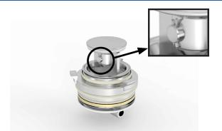
Dismounting the inner package by removing the pin and splint (pos 5 & 63) from the piston. Remove all parts from the inner package in order to change the seals (pos 8 & 77) on the driving plate and the seal (pos 3) on the piston.
