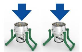
Assemble the shaft and two rollers for piston guide by applying pressure to the driving plate packet.
