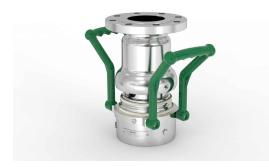
Remove the swivel sleeve by pulling out the hose unit body with the inner package. If the swivel sleeve cant be removed, there might be some balls left inside. Try turning back and forth again to get out the remaining balls.
