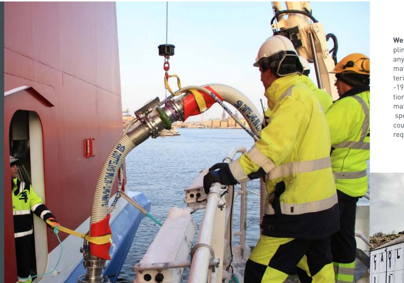
We design the widest range of DDC couplings in the world – available in almost any existing metal and many composite materials. Combined with sealing materials with working temperatures from –196°C to +280°C, and the largest variation of connections, this makes a unique match to specific requirements. To fulfil special handling procedures our couplings could be equipped to suit almost any requirements.
