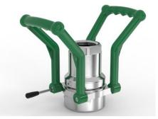
Unscrew and remove the lock screw (pos 23) and o-ring (pos 78) from the swivel sleeve.
