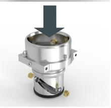
Put a shaft into the piston guide (pos 7) and turn the driving plate to the position where the driving plate heels are coming free from the rollers. It could be necessary to release the package from the press force.
