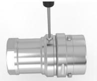
Put a small container underneath the coupling and start twisting the swivel sleeve, so the balls drop out, into the container. Placing a tank unit in the hose unit will make it easier to twist. Clean and save the 41 balls for reassembling later.
