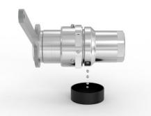
Remove the swivel sleeve by pulling out the hose unit body with the inner package. If the swivel sleeve cant be removed, there might be some balls left inside. Try turning back and forth again to get out the remaining balls.
