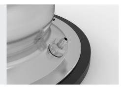
Change the O-ring and test if the Perc valve is rotating without problems.
